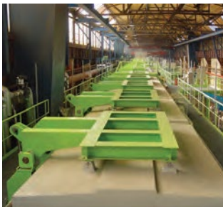
Plating and pickling tanks, covers: SIMONA® PP
