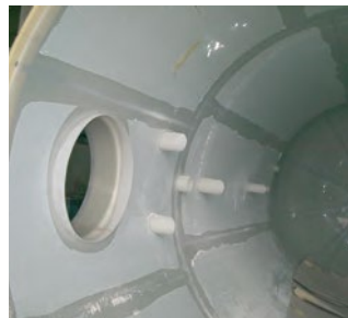
Dual laminate process tanks: SIMONA® PVDF 740 fabric backed
